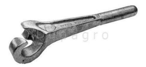
TITAN "100 SERIES" VALVE WHEEL WRENCHES are made from aluminium-magnesium to reduce the chance of sparks when opening stubborn valves.
